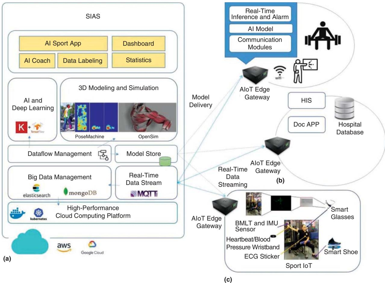
**FIGURE 1.** The AIoT sports science system architecture. (a) The SIAS. (b) The AIoT edge computing configuration. (c) The sport IoT system at the training equipment. HIS: health information system; IMU: inertia measurement unit; Doc: doctor.
