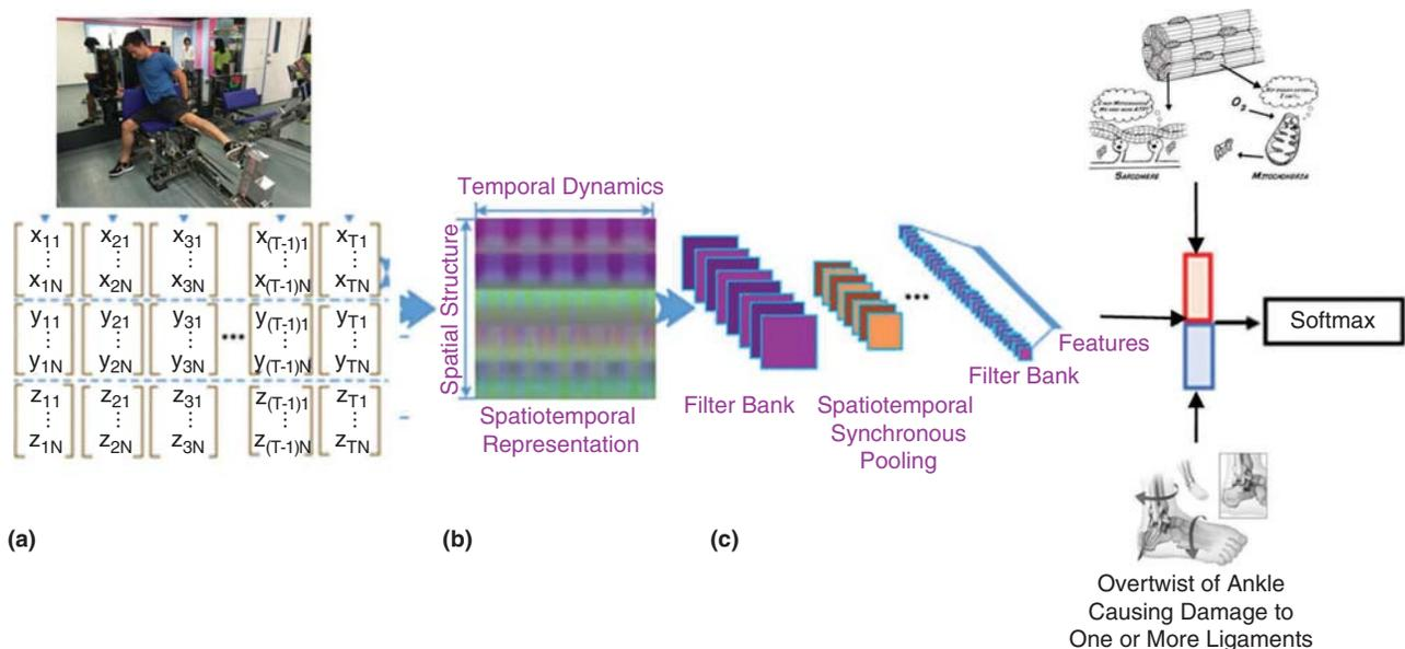
**FIGURE 6.** The process for CNN training and fatigue pattern labeling. (a) A matrix of values recorded from the joint coordinates forming the skeleton structure. (b) A spatiotemporal image matrix from a sequence of motion over a training period. (c) The resulting softmax weighting matrix after pooling with the CNN.
